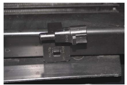
Position the sensor with the mounting flange on top of the cross member. Use a pen to mark where the new hole will be drilled. Make sure the wiring harness is able to connect to the senor in its new position. Set the sensor aside and drill a 1/4" hole to accommodate the new plastic push-in fastener. Reconnect the wiring harness to the sensor and install the push-in fastener. Continue with grille assembly installation from Step 7.
