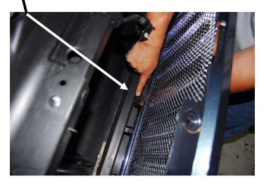
7. Start the installation of the completed mesh grille panel by snapping in the (4) fasteners on the bottom of the grille panel. Apply pressure to the outside of the grille panel until all (4) fasteners have snapped into place.
