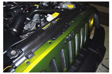
8. Reconnect the turn indicator lamp wires and position the grille panel so the upper holes align with the holes in the upper support. Install (6) supplied Push-In plastic fasteners in the same holes that the originals were removed from.
