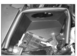
18. Install the heat shield assembly into the engine compartment and secure with the three bolts removed in step #12.
