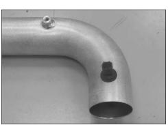
8. Install the air temperature sensor into the grommet installed into the K&N intake tube during step #6.
