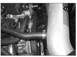
20. Connect the crank case vent hose to the K&N intake tube and secure with the provided hose clamp as shown.
