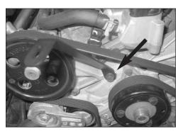
11. Install the supplied tube mounting bracket (26653) onto the engine and secure with the bolt removed in step #10. NOTE: Be sure the bracket sits flush to the engine.
