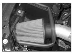
21. Install the K&N air filter and secure with the provided hose clamp.
