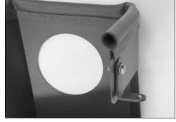
16. Install the supplied "L" bracket (070812) onto the heat shield as shown with the provided hardware.
