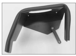
15. Install the supplied bracket (07097) onto the rubber mounted stud as shown. NOTE: Do not completely tighten at this time.
