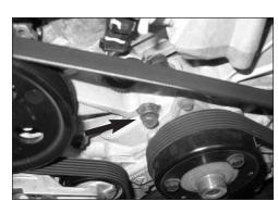
10. Remove the front engine bolt shown. NOTE: This bolt will be reused.
