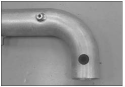
6. Install the supplied grommet into the hole in the K&N intake tube as shown.
