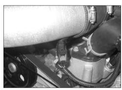
22. Reconnect the air temperature sensor electrical connection.
