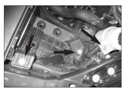
12. Remove the power steering reservoir mounting bolt and the two air box bracket mounting bolts shown.
