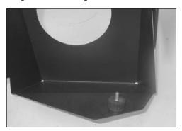
14. Install the supplied rubber mounted stud onto the heat shield with the provided hardware as shown.
