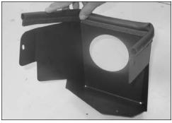
13. Install the supplied edge trim onto the heat shield as shown.
