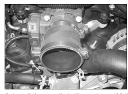
9. Install the supplied silicone hose (08173) onto the throttle body and secure with the supplied hose clamp.
