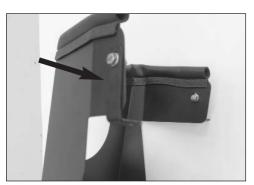
17. Install the supplied "L" bracket (07195) onto the heat shield as shown with the provided hardware.
