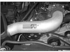
19. Insert the K&N intake tube into the silicone hose at the throttle body and align with the mounting bracket installed in step #11 and then secure with the hose clamp and hardware provided.
