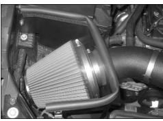
24. Install the K&N air filter assembly on the K&N intake tube and secure with the provided hose clamp as shown.
