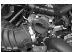
4. Loosen the hose clamp that secures the stock intake tube to the throttle body and then disconnect the intake tube from the throttle body.
