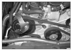
12. Install the tube mounting bracket assembly onto the engine and secure with the bolt removed in step #10.
