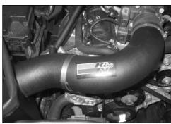
20. Insert the K&N intake tube into the silicone hose at the throttle body and align with the mounting bracket installed in step #12 and then secure with the hose clamps provided.
