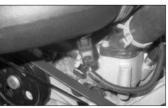
25. Reconnect the air temperature sensor electrical connection.
