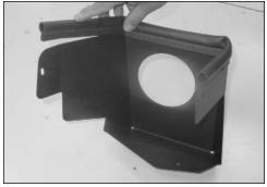
14. Install the supplied edge trim onto the heat shield as shown.
