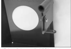
17. Install the supplied "L" bracket (070812) onto the heat shield as shown with the provided hardware.
