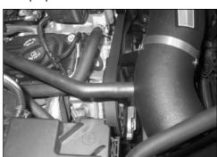
21. Connect the crank case vent hose to the K&N intake tube.
