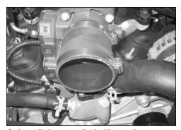
9. Install the supplied silicone hose (08173) onto the throttle body and secure with the supplied hose clamp.
