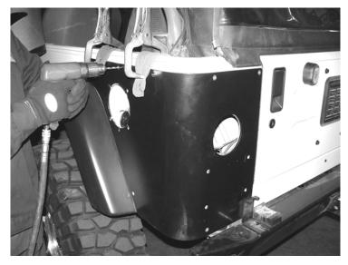
4. Install the supplied Counter-sunk Torx bolts. Install nylock nuts, and washers to ALL EXPOSED BOLTS ON THE INSIDE OF THE JEEP. The self-threading bolts are ONLY to be used WITHOUT the nylock nuts where there is no access to the backside of the bolt. Do not over tighten the bolts where a nylock will not be used. SEE PHOTO BELOW.
