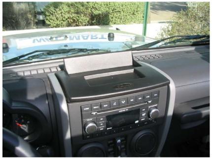
7. Using a philips screw driver install compass module onto the Daystar panel.
