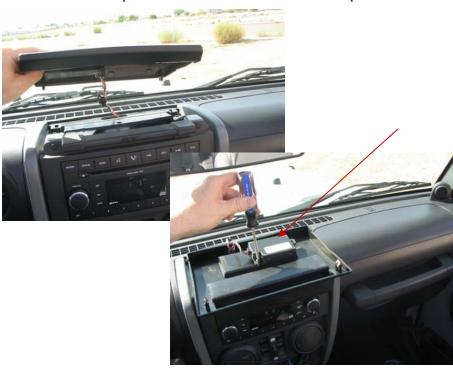
4. Using a flat head screw driver remove the 2 clips.
