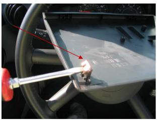
5. Using needle nose pliers compress the clips so they will clamp on the Daystar panel.
