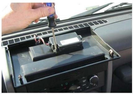
8. Rotate the panel over so you can install the panel from the front down so it will catch the dash first.
