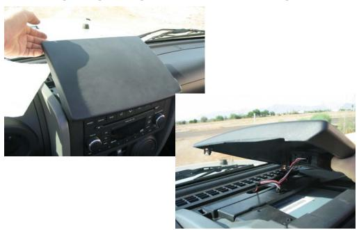
3. Turn the panel over , using a Philips screw driver , remove the 2 screws that holds the compass module and remove the module from panel.
