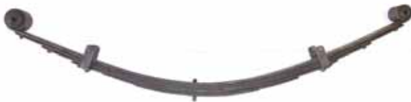
< FRAME END (LARGE BUSHING) – PHOTO 3 – SHACKLE END >
