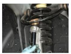
10. Lower the floor jack to relieve all spring tension and remove the lower strut mounting bolt where it mounts through the lower control arm.
