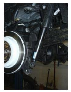
6. Install the upper coil spacer along with the isolator pad and bumpstop cup removed in step 5. Use the longer bolt provided in the kit - 10 mm x 75 mm long.
