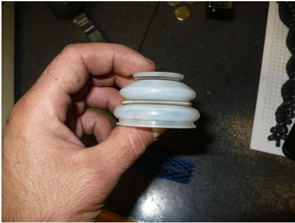
9. Install dust boot onto tie rod end and roll lower spring down to the bottom lip of the dust boot as pictured below.
