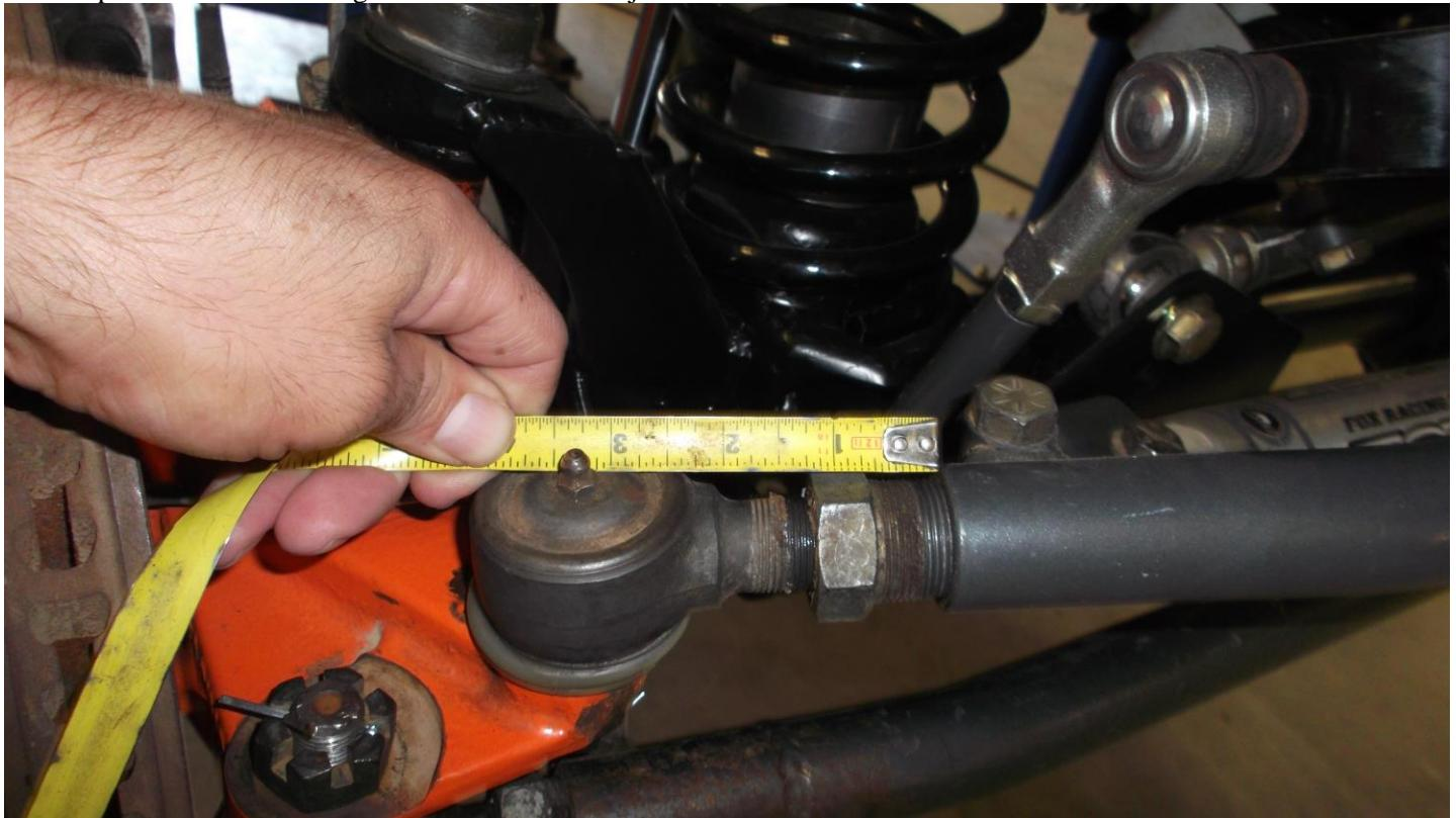
15. At this time, fully tighten the jam nut at the pitman arm side. Really crank this down as jam nuts tend to loosen up if not fully tight. Also, do not forget to install the cotter pin at the pitman arm side.
