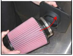
11. Place the S&B filter assembly into the S&B air box. Once the filter is inside the box tilt the adapter back so as to catch the hook on the bottom, then secure with the 5/16 screws (F).
