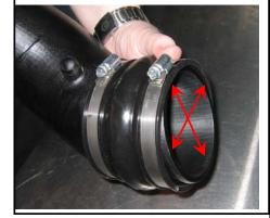
17. Install S&B tube (J) into the step adapter (M) at the throttle body. Center the hump adapter IH) over gap between tube ends and secure both #72 hose clamps (H), then secure # 52 hose clamp (L) at the throttle body end.
