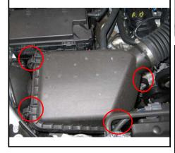
5. Pull up on the OE air box to remove it from the vehicle, there are 3 barbed prongs seated in rubber grommets on the bottom side.
