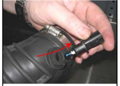
15. Install the S&B step adapter (M ) over the throttle body and secure the # 52 hose clamp (L).
