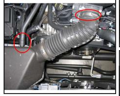
4. Unclip the air box lid and remove the lid and tube assembly from vehicle.
