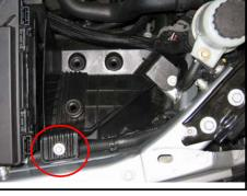
8. Place the S&B air box (A) in the vehicle, insert prongs into OE grommets and push the bottom downward to seat the prongs.
