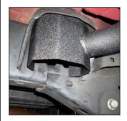
**Step 3.** Supporting the RRC Side Armor from underneath, lift the Armor into place and slide it between the large washer and the body mount, taking care to align the holes in the Armor mount with the two body mount studs. Apply several drops of the included threadlock to the studs. Thread the two nuts onto the studs loosely. Repeat for each body mount location.
