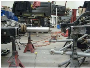
12. Locate the frame sleeves. Use a small tack weld to locate the frame sleeves half way into the frame openings. Remove any E-coating where the sleeves will be welded or tack welded prior to placing them into the frame.
