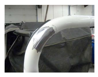
5. Cut the rear seatbelt supports off of the sport bar. Unbolt the rear and discard. Using a grinder, sanding disc and ScotchBright pad, clean up the intersection of the sport bar and rear seatbelt support bar to a polished finish.
