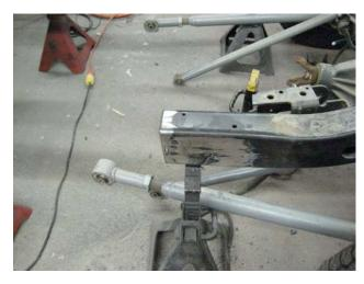
11. Prep the frame ends for welding. Carefully clean all slag or burs from inside the frame rails with a file or die grinder. Using the four inch angle grinder bevel the edges of the frame rails with a 45 degree angle.
