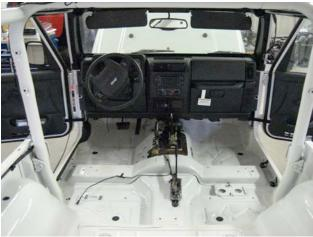
10. Clean up the tub. Using a hammer and dolly along with the wire brush and sanding discs, clean up all the separated areas. Remove all paint and excess seam sealer. Straighten any bent edges and remove any burs leftover from drilling the spot welds out. You are now done with the Body tub preparation.
