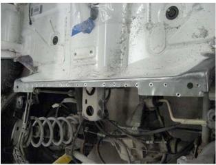
11. Remove the front half of the Jeep body from the frame and set it aside. Its time to prepare the frame.
