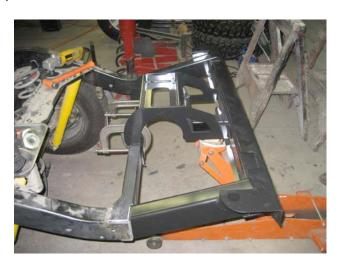
3. Check the location. Using a long straight edge, check the height locations of the body mount surfaces as shown. Check for squareness and overall length. Once you are satisfied with the position of the Rear Frame Extension, clamp everything down tightly and re-check all your measurements.
