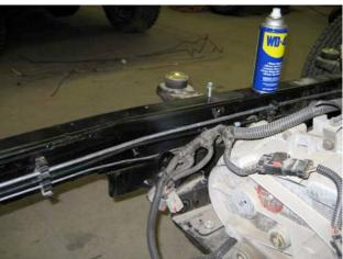
7. Install the E-brake cables. Install Jeep Unlimited E-brake cables; part #52013455AB & #52013457AB for disk brakes. For drum brakes and custom applications we have found the Lokar Universal Emergency Brake cable to be easy to adapt to the Wrangler's bracket and lever.
