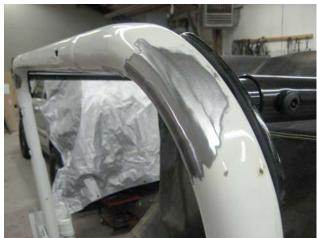
6. Mark all the spot welds to be cut. Use a spring loaded punch, *carefully* mark the center of each spot weld. This is another area where taking your time will save you aggravation later. Precisely marking the center will ensure that you cut the entire spot weld out in step 7. If you do step 6 and 7 accurately, the panels will separate cleanly and easily. Mark the welds in areas A,B,C,D,E.
