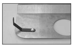
16. Install the provided "C" bracket (#07171) onto the heat shield with the provided hardware as shown.
