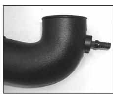
26. Install the ¼" NPT fitting into the K&N<sup>®</sup> intake tube as shown.
