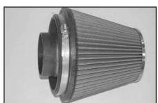
30. Install the air filter adapter into the K&N® air filter and secure with the provided hose clamp as shown.
