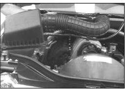
6. Remove the upper air box housing and intake tube assembly as shown.
