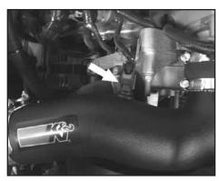
29. Re-connect the air temperature sensor electrical connection.
