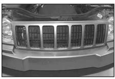
33. Re-install the grille assembly and secure with the factory retaining clips.
