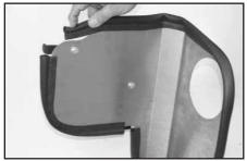
20. Install the long edge trim onto the heat shield assembly as shown.
