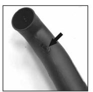
25. Install the air temperature sensor into the grommet installed into the K&N® intake tube in the previous step.
