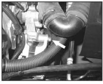
14. Remove the upper alternator mounting bolt as shown.
