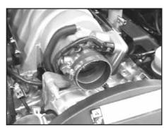
22. Install silicone hose (#08630) onto the throttle body and secure with the provided hose clamp.
