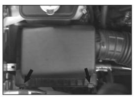
5. Release the two air box clam shell clips as shown.
