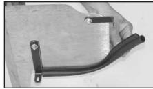
19. Install the short edge trim onto the heat shield assembly as shown.
