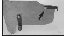
18. Install the small "L" bracket (#07158) onto the heat shield with the provided hardware as shown.
