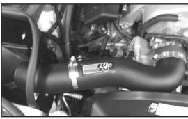
27. Install the K&N® intake tube into the silicone hose on the throttle body and align with the saddle clamp. Then, secure the intake tube with the provided hose clamps.
