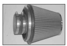
31. Install silicone hose (#08630) onto the K&N® air filter assembly and secure with the provided hose clamp.
