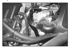
15. Install the tube mounting bracket assembly onto the upper alternator mount using the bolt removed in the previous step.
