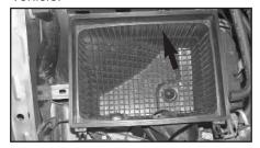
10. Remove the air box mounting bolt as shown.
