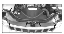
8. Remove the six grill retaining clips from the grille. Then, tilt the grille forward and lift, removing it from the vehicle.
