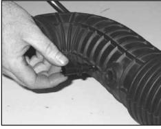
23. Remove the air temperature sensor from the stock intake tube as shown.
