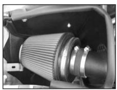
32. Install the K&N® air filter assembly onto the K&N intake tube and secure with the provided hose clamp as shown.
