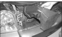
9. Pull the fresh air duct forward to disconnect it from the air box, then remove it from the vehicle
