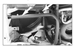
21. Install the heat shield assembly into the vehicle. Secure to the lower and upper air box mounts and washer bottle stud with the provided hardware.
