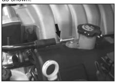
3. Disconnect the crank case vent from the valve cover as shown.
