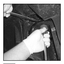
1.6 Tighten the top nut on the shock. Holding the shock shaft should be sufficient, but again, you may use a wrench on the hex on the shock shaft if necessary.
