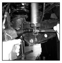
Install the bottom of the new shocks into the housing bracket and affix them using the factory bolt and nut.
