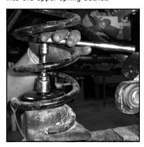
Put blue loc-tite on the 1/2''- $13 \times 1''$  bolts before installing them, and then tighten them down.
