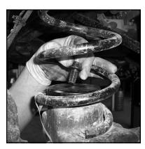
NOTE: Make sure the end of your spring is indexed into the stamped groove in the housing pad correctly! Now install the bumpstop spacers - countersunk hole side up!
