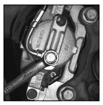
Now go back and tighten the banjo bolts on the calipers - observing the location of the bends in the ends of the hoses.
