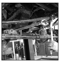
Next step is to reinstall the trac bar bolt. This may require the use of a come-along to realign the bolt hole. After you get the bolt in put the nut on the back of it, but do not tighten it!
