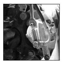
Crack both bleeders on the calipers to gravity bleed your brake system. Fluid will flow out of them one at a time when they are bled. As soon as fluid flows out, close the bleeder.
