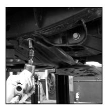
6 Remove all of the transmission skid plate bolts except the end one on the passenger side. Loosen this bolt and leave it in to allow the plate to hang out of the way for the rest of the job.
