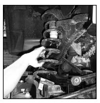
Next, release the jack load under the frontend housing to lower the frontend. This should allow you to easily remove the front coil springs.
