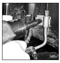
Remove the bolts that hold the brake hose tabs to the frame. Save these bolts for reuse! You may now remove the hoses from the vehicle.
