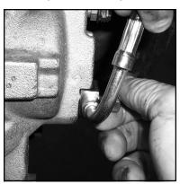
Put the banjo bolts through the ends of the new hoses, put the other 2 washers on, and then start the banjo bolts into the threads in the calipers. Do not tighten.
