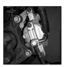
Next remove the banjo bolt from the caliper. Be prepared! Fluid will come out!
