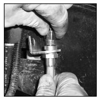
With the new frame tabs already slid onto the new lines' fittings, you may attach the brake hard lines into the new brake hoses. Do not tighten the fitting!
