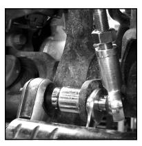
The lower stud on the link goes in the bracket from the engine side of the bracket - nut on the tire side of the bracket! Start the nut onto the stud - but do not tighten!
