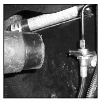
Finally, go back and install the brake line fitting to frame tab clips with a mallet. Your brake line installation is now complete.
