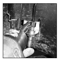
Attach the new frame tabs to the frame with the factory bolts that you took out in step 25.
