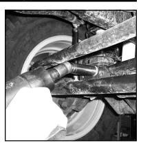
Put the tires back on the vehicle and set it back on the ground. Now you may go back and tighten the trac bar bolt.
