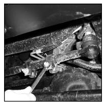
Your steering will require a minor adjustment by a competent alignment shop. This issue must be addressed! If your steering wheel is not straight the vehicle ESP system can mistakingly sense that the vehicle is in a turn and apply the brakes!
