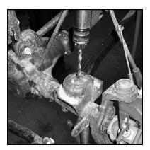
With a 7/16" drill bit, drill a hole in the center of the coil spring pad on the frontend housing.
