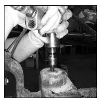
Install the thread-forming 1/2"-13 x 1" long bolts into the holes. After the bolts have tapped the holes with threads - take them back out of the holes.
