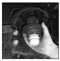
Pull the stock rubber spring isolater pad down off of the upper spring bucket on the frame.
