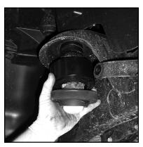
Install the RockJock coil spring spacer - chamfered lip side DOWN - and the stock rubber isolater pad back into the upper spring bucket.
