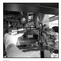
Jack the vehicle up and set it on jackstands by the frame, and then with a jack under the frontend housing, raise the housing to a height that relieves the load on the sway bar. Remove upper sway bar link ends from the sway bar.
