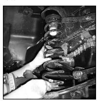
Reinstall the coil spring against the isolater and spacer, and then index the bottom of the spring back onto the spring pad on the housing.
