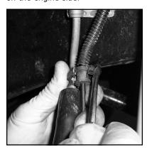
Pull all the plastic clips off, releasing the wires from the hoses.
