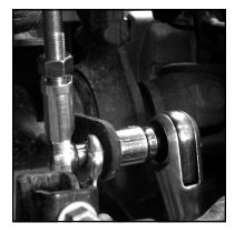
Next you may now go back and tighten the nyloc nuts on the housing end of the sway bar links. This will require 2 wrenches or a wrench and a socket.
