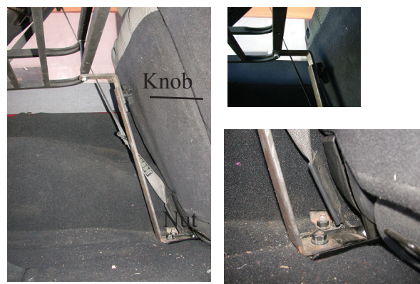
Two piece Z Bar mounting bracket. With quick disconnect knob.
