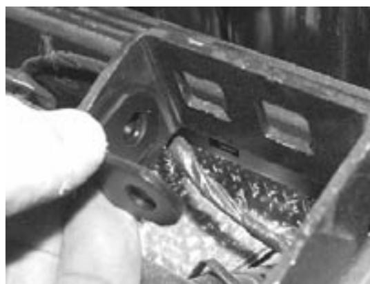
Take the end of the cable and run it through the top of the thumb lever down through the boot then through the center console.
