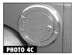
**4.** Take the supplied self tapping screws and insert them through the fuel door brackets into the fuel bucket using a 1/4" nut driver (See Photos 4A & 4B). You are now finished (See Photo 4C).
