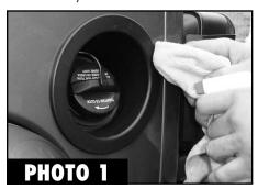
1. Extremely Important: Clean the area where the Fuel Door is to be installed. If the area where the Fuel Door is to be installed is not clean, dry, and free of any vinyl dressing, the Fuel Door will not stick in place. Begin by cleaning the area thoroughly with a good non-residue cleaner such as Windex, or just clean thoroughly with soap and water and dry completely.
