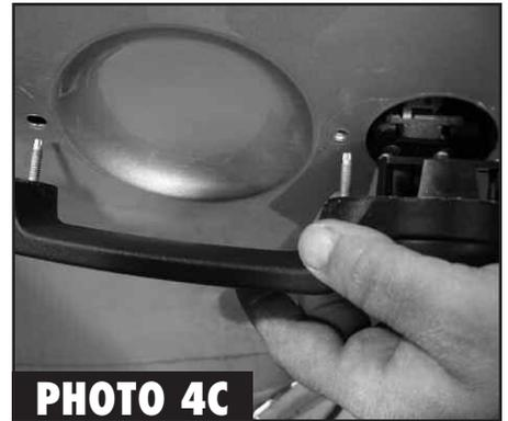
**4.** Remove both nuts using a 5/16" socket and ratchet. A swivel may make the process easier (See Photo 4A & 4B). Hold the handle from the outside of the door to prevent falling and remove (See Photo 4C).
