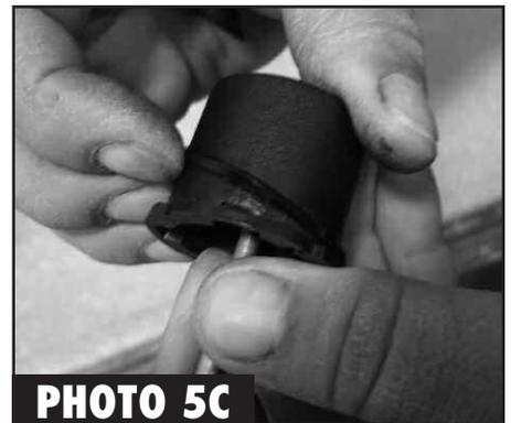
**5.** With the handle face down on a workbench, remove the two torx screws with a T-10 torx driver (See Photo 5A). You can now remove the plastic mounting clip and spring from the factory handle (See Photo 5B). Now take out the push button and remove the plastic spacer (See Photo 5C).
