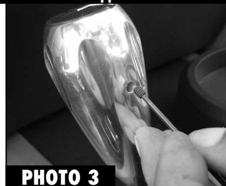
Begin by setting the parking brake, placing the transmission in natural, and put the transfer case in natural or 4lo. With a firm pull, the stock shifter will come off (Photo 1). Place your new Billet Shifter into place and align for the set screw (Photo 2). Insert the set screw into the V-shape portion of the shaft and tighten (Photo 3).
