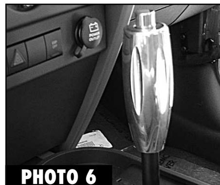
Begin by twisting the bottom boot of the shifter clockwise (Photo 1). Remove the torx head screw with a t-20 torx (Photo 2) and pull the stock shifter off (Photo 3). Place your new Billet shifter back in place (Photo 4). Align the set screw back up and tighten (Photos 5 and Photo 6).
