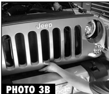
**3B.** Repeat this on the other side then pull outwards towards the center removing the last 4 clips. (See Photo 3A)
