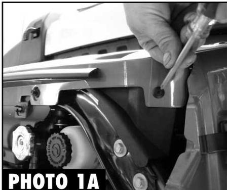
**1.** Begin by removing the front grille. Start by opening the hood and removing the six factory clips. Using just a Phillips head screwdriver, loosen and remove all six clips. (See Photos 1A & 1B)
