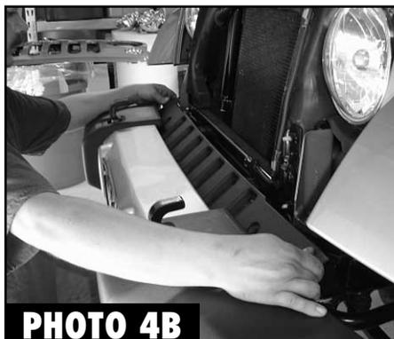
**4B & 4C.** Remove the bumper spacer plate. (See Photos 4B & 4C)
