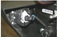
Plug the fog lamp wiring back into the installed fog lamps.
