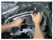
**NOTE:** Verify that the long side of the mode sleeve is towards the front of the transfer case.
