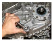
4.Loosen the rear case with a pry tool to break the bead of sealant between the cases
