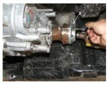
3. Use a 32mm socket and an impact wrench to remove the 22mm flanged nut from the rear output yoke. If you do not have an impact wrench it will be necessary to hold the yoke as you loosen the nut.
