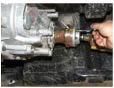
2. Using an 8mm socket remove the [8] 8mm bolts (#1) from the rear output flange and disconnect the rear driveline. Support the driveline out of the way to avoid damage to the CV joint that is still attached to the rear differential, or repeat the steps 5 and 6 and remove CV joint from the rear differential.
