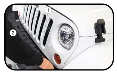
2. Remove the font splash shield (3) by removing the 4 push pin fasteners(1) connecting it to the bumper the 2 push pin fasteners (4) that connect it to the frame behind the splash shield.
