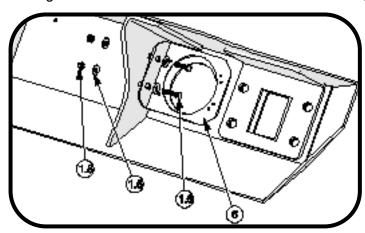
remove the 8 nuts that attach the studs from the bumper to the frame. Slide the front cross member decorative cover to gain access to the nuts.
