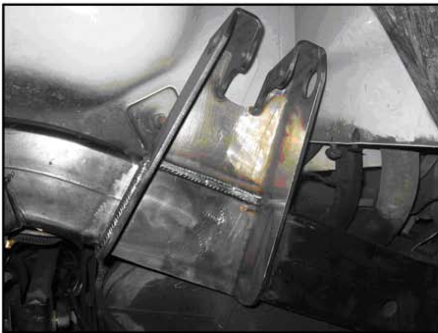
Weld completely around the upper shock mount
