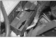
4. Disconnect the vacuum canister hose shown.
