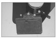
18. Using the provided spacer, install the vacuum reservoir onto the heat shield as shown. NOTE: Due to vehicle manufacturing tolerances, 2 spacers may be required.
