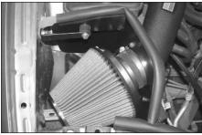
29. Install the air filter assembly onto the K&N intake tube as shown and secure with the povided hose clamp.
