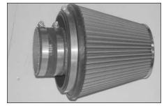
28. Install the silicone (08630) onto the air filter assembly and secure with the provided hose clamp.
