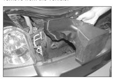
7. Pull the fresh air duct forward to disconnect it from the air box and then remove it from the vehicle
