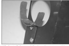
12. Install the saddle bracket assembly onto the heat shield with the provided hardware as shown.
