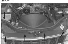
5. Using a small screwdriver, release the center holding pins in the six grill retaining clips
