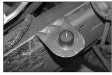
20. Using the two fender washers and one rubber washer, install the 6mm male/female rubber mounted stud onto the lower air box mount as shown
