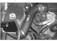
25. Install the K&N intake tube into the silicone hose at the throttle body and onto the saddle clamp, then secure with the provided hose clamps as shown.
