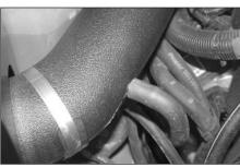
26. Connect the crank case vent hose onto the K&N intake tube as shown.
