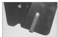
13. Install the "L" bracket (070952) onto the heat shield with provided hardware as shown. NOTE: Mount this bracket on the inside of the heat shield with the "L" pointing to the outside.
