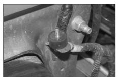
21. Install the 6mm male/male rubber mounted stud onto the upper air box mount as shown.
