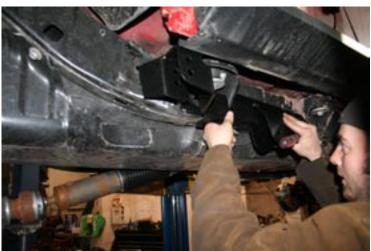
6. Use a heat shield as shown in the photo below to protect the fuel tank during final grinding and installation and welding of the new right rear long arm bracket.
