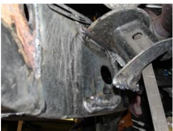
3. Remove both front upper and lower brackets and grind the remaining weld smooth with the frame in preparation for installing the new combination front bracket. The new front bracket mounts to the cross member bolts, locates to an existing hole in the frame with a single bolt up through the bottom of the frame (some models may not have threads in this frame hole). Push the new bracket up tight against the frame before welding in place.
