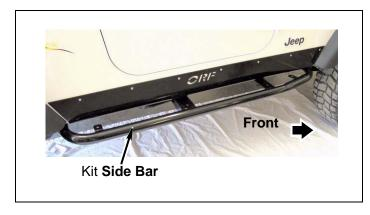
6. Fasten kit **side bar** to **ORF rocker panel** with two kit **bolts** (3/8" x 1") and **washers** (3/8" USS). DO NOT tighten.
