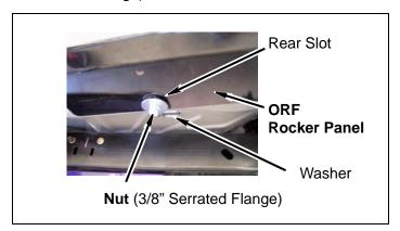
5. Install kit side bar between washers (9/16" ID x 2" OD) and ORF rocker panel.
