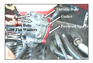
**4.** Install the Poweraid Spacer (#1) with the bore extending into the intake manifold. Install the Gasket (#2) between the Poweraid Spacer and the throttle body. Install four 6mm x 50mm hex bolts (#3) and 6mm flat washers (#4) through the throttle body, Poweraid Spacer, Gasket, and into the intake manifold. Using a 10mm socket, tighten all four throttle body bolts evenly, to the manufacturer's specifications. **Do Not Over Tighten The Bolts!**
