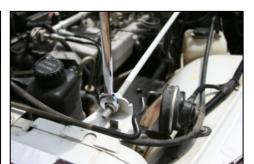
**5.** Using a 10mm socket, remove the horn bolt. (Save for later use.)
