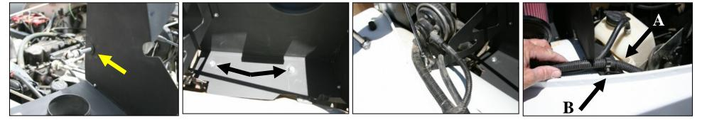
**9.** Carefully slide the CAD over the support rod, and then slide the supplied grommet over the rod, and into the hole in the CAD as shown. Rotate the CAD and place into position on the factory airbox mount. Reinstall the radiator support rod, and tighten the nut.
