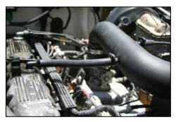
**17.** Replace the factory breather hose with  $\frac{1}{2}$ "x10" rubber hose between valve cover and intake tube using speed clamps as shown.
