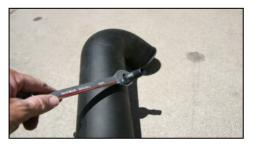
**14.** Install the  $\frac{1}{4}$ " barbed fitting into the intake tube.
