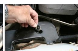
**4.** Remove the two grommets from the airbox mounting plate.
