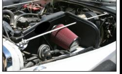
**18.** Install the Airaid Premium Filter and the weather strip on the CAD, as shown. (Hint: start the weather strip near the radiator support and work towards the back of the vehicle.)
