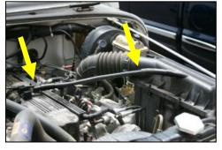
**1.** Disconnect negative battery cable. Remove factory valve cover breather hose from airbox, and valve cover.
