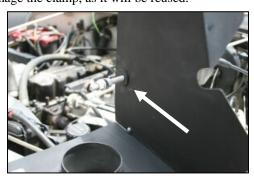
**9.** Carefully slide the **CAD** over the support rod, and then slide the supplied grommet over the rod, and into the hole in the **CAD** as shown. Rotate the **CAD** and place it into position on the factory airbox mount. Re-install the radiator support rod, and tighten the nut.
