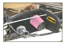
18. Install the Airaid Premium Filter (#1)and the weather strip (#9) onto the CAD, as shown. Apply the Airaid Foil Decal onto the Panel as shown.
