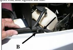
12. A) Using a ¼-20 bolt (#13), 2 washers (#14), and locknut (#16), bolt the CAD to the fender. B) Install the wire loom clamp into the hole in the CAD, as shown.
