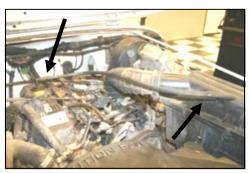
1. <u>Disconnect the negative battery cable.</u>
