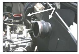
**15.** Install the urethane hump hose (#6) on the **CAD** with two #60 hose clamps (#18), and the coupler (#7) on the throttle body with two #44 hose clamps (#17). Leave the clamps loose for now.
