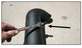
14. Install the 1/4" barbed fitting (#22) into the intake tube.
