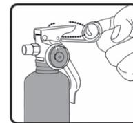
1. HOLD EXTINGUISHER UPRIGHT AND PULL THE RING (SAFETY) PIN
