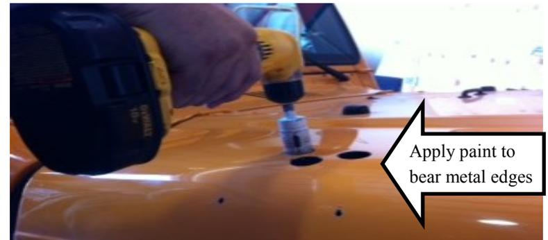
10. Deburr the holes drilled in the steps 8 & 9 and use some touch up paint on bear metal edges to prevent corrosion.
