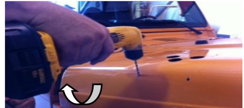
9. Change over to the 1-1/4" hole saw and cut out the three (3) vent holes.
