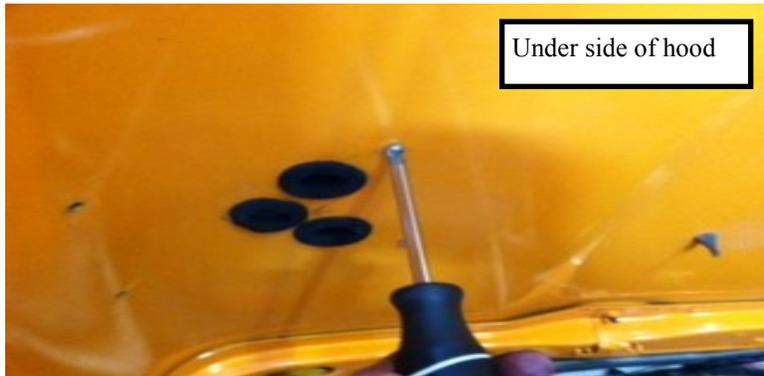
15. Starting with the 3/16" long bolts, secure the Daystar hood vent to the hood.
