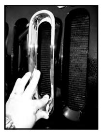
3. Clip lower retainers behind grille shell, and then push the top in until it clips in place. This usually can be accomplished by simply pushing on the insert, but sometimes it is helpful to squeeze the insert to the grille shell as shown.
