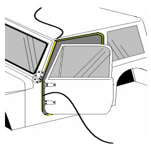
Over time door hinges will wear and cause air to leak between gaps in the door seals. Shimming, realignment, and or possible bending of the top window frame towards the top might be needed for a better seal. If leaks are not corrected wind noise may develop.
