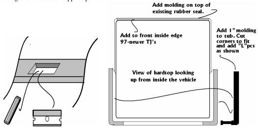
Cut the corners to fit and add the small "L" side pieces as shown. Be sure to cut the four holes on each side using a razor blade or supplied punch. (3 holes for TJ's).
