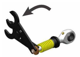
• Slide the spring off of the shaft.
