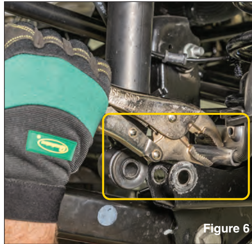
Using locking pliers, separate the bracket from brake line (FIGS 6 & 7).
