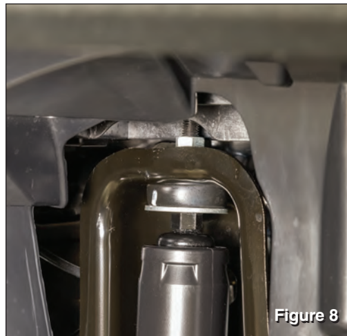
Remove original equipment front shock absorbers. Locate the shocks fasteners as shown.
