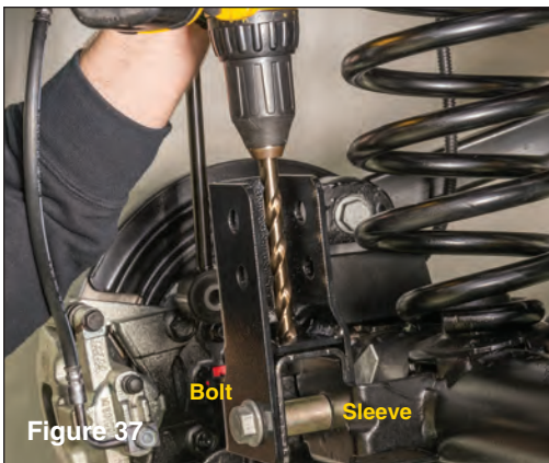
Figure 37 Place supplied rear track bar bracket over axle housing. Install OEM bolt and crush sleeve, but do not tighten at this time. Carefully drill a hole through the track bar bracket into axle housing bracket as shown using a 15/32 " drill bit. Consider drilling pilot holes. (see FIG 37)
