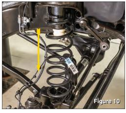
Gently lower axle housing towards the ground and remove original coil springs. (see FIG 10)
