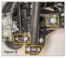
Moving to the rear of the vehicle: Raise rear end and properly support using jack stands. Disconnect the rear track bar bracket from axle using 21mm socket, remove rear lower shock bolts and sway bar end links using a 18mm socket & open end wrench (see FIG 18).
