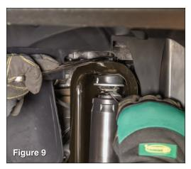
Disconnect the top end of the front shocks using an 5/8" open end wrench. (see FIG 9)
