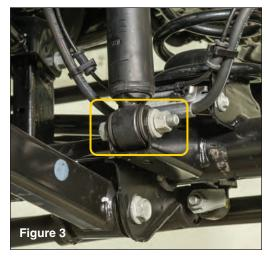
Disconnect the bottom end of the front shocks using an 18mm socket and open end wrench. (see FIG 3)
