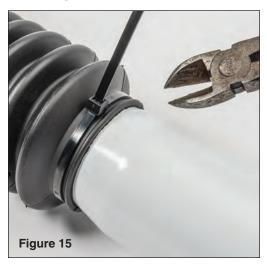
Assemble your new front shocks as shown in FIG 15, 16 &17. Install the shock boots and secure with zip-ties. Clip off zip-tie tail.
