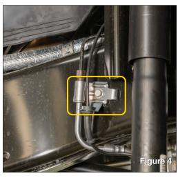
Disconnect brake line bracket from frame using a 10mm socket. (see FIG 4)
