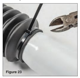
Assemble your new rear shocks as shown in FIG 23, 24 & 25. Install the shock boots and secure with zip-ties. Clip off zip-tie tail. (see FIG 23).
