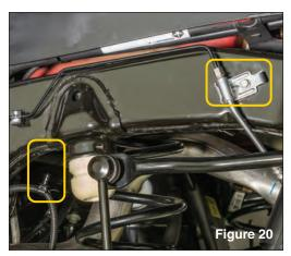
Disconnect ABS line from frame and disconnect brake line from frame using a 10mm socket. (see FIG 20)
