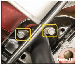
Now disconnect the top end of the rear shocks using a 16mm socket as shown above (see FIG 19).
