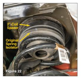
Lower axle down and remove factory rear coil springs. Install new 2" coil spacer on top of the original equipment spring isolator (see FIG 22).
