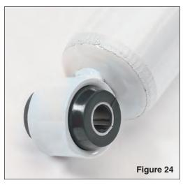
Assemble the shock bottom bushings exactly as shown (see FIG 24).
