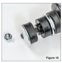
Assemble the shock top bushings exactly as shown (see FIG 16).
