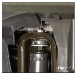
Remove original equipment front shock absorbers. Locate the shocks fasteners as shown.
