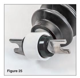
Push the mounting plate with bushing through the top eyelet of the rear shocks (see FIG 25).
