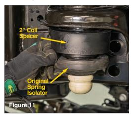
Remove factory coil spring isolator and place provided 2" coil spacer on top of Original Equipment spring isolator, exactly as shown (see FIG 11). Locate the new front bump stop in the kit.
