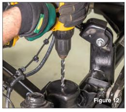
Using the bump stop as a template, mark the center of the bump stop pad located on the front axle. Consider drilling pilot holes. Carefully drill the bump stop pad using a <sup>25</sup>/<sub>64</sub>" drill bit. (see FIG 12)
