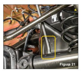
Disconnect axle housing vent line. (see FIG 21)
