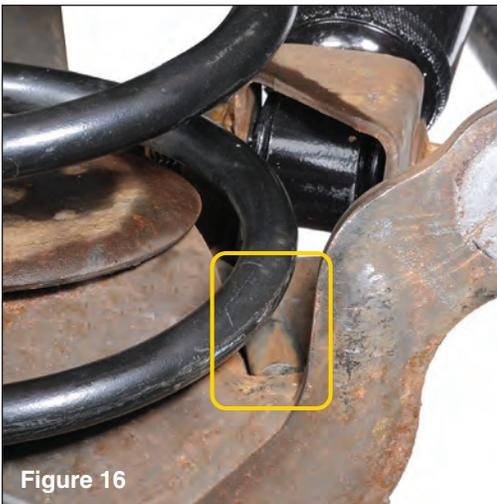
Install new coil springs and index on bottom mount as shown (see FIG 16) Carefully raise axle enough to re-attach the control arm to frame using original bolt. Install bolt and nut loosely at this time.
