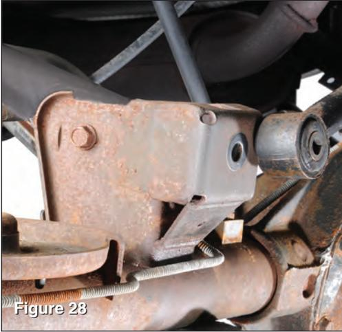
Locate rear upper axle control arm mounting bolt and remove using a 15mm socket and open end wrench. (see FIG 28)
