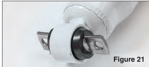
Locate and assemble front shocks as shown (see FIG 20 & 21). Install into original opening at top mount and torque to 20 ft. lbs. using a 9/16" socket.
