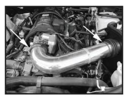
Step 19 Install the intake tube into the flex coupler first then into the coupler on the throttle body. Once in the desired location fasten it securely in place.
