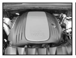
Step 2 Start by removing the engine cover that is attached by small ball and socket joints.
