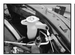
Step 13 Remove the center pin using a screwdriver to help remove the center pin. Once the center pin is removed, remove the panel clip from the vehicle. This will be reinstalled in a later step.
