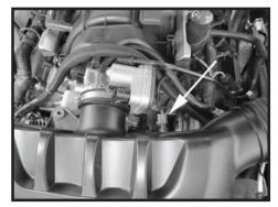
Step 4 Disconnect the electrical connector on the Intake Air Temperature (IAT) sensor.
