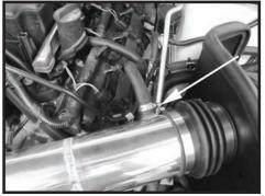
Step 20 Reconnect the factory breather line to intake tube and fasten it securely in place with the supplied clamp.
