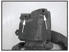
Step 10 Remove the factory grommet from the air box. This will be reused on the next step.
