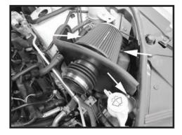
Step 16 Install the heat shield assembly in the vehicle. Align the grommets onto the pins located on the inner fender as well making sure the bracket is on the flex coupler side of the heat shield.
