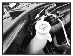
Step 15 Install the bracket with bolt removed in the previous step. The large hole is used to mount the bracket to the core support.
