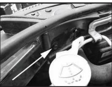
Step 14 Remove the bolt on the core support. This will be reused in the next step.
