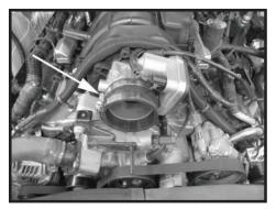
Step 18 Install the coupler on the throttle body and secure the boot in place. Install a second clamp but do not tighten at this time.
