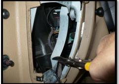
**'97-'00 models** must remove the section of metal bracket on the driver and passenger sides...
