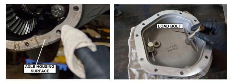
11. Install the rest of the supplied bolts and washers and torque to 15 ft/lb. in a crisscross pattern.
