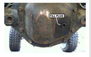
4. Carefully pry the cover loose with a flat head screw driver, being careful not to damage the surface, and allow the oil to drain.
