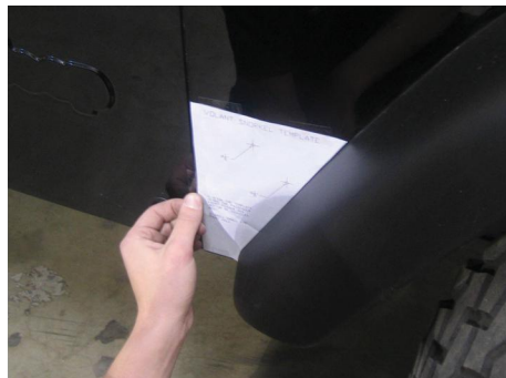
2. Align template along the side base of the jeeps passenger fender. Tape the template to the fender.
