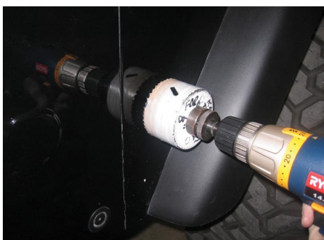
4. Remove the template from the fender. Drill a 3" hole with a hole saw on the top 1/8" pilot hole and a 3/8" hole with a drill bit on the lower pilot hole.
