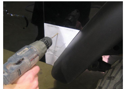
3. Once the template is lined up and taped to the fender, drill two 1/8" pilot holes as noted on the template.
