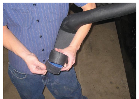
6. Place the 3" X 3" sleeve on the small opening of the Volant down pipe and the 3/4" X 2" sleeve on the other end of the short snorkel..
