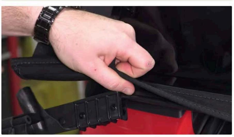
Now the tailgate bar will lock into the two tailgate brackets you installed earlier on the body tub.
