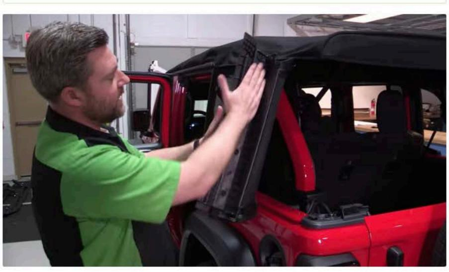
The Rear window will install the same way as the top of the side windows. Just slide the window into place.
