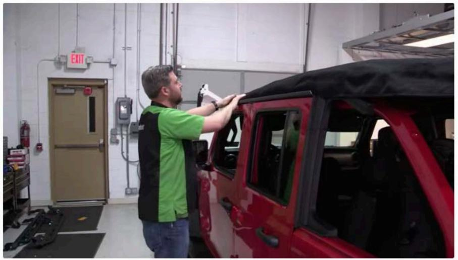
Grab the windows and slide them into place. There is a bead on the top that the window channels will slide into.
