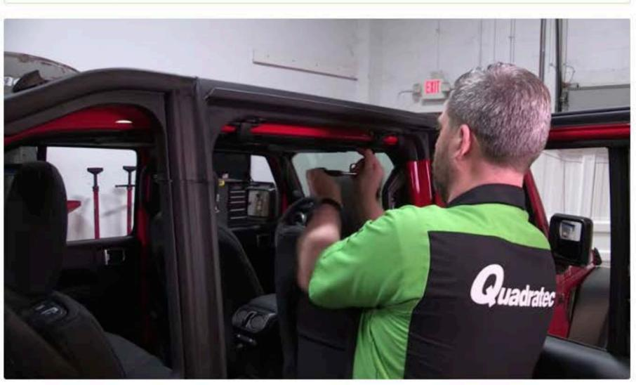
Next you are going to attach the soft top portion. You can leave the protective cover and straps on until you get the top situated on the back of the Jeep, this will make it easier to move around and handle.
