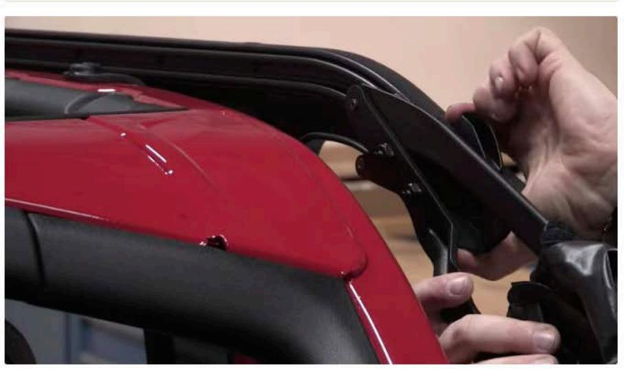
Now you can go ahead and remove the protective cover. The last thing you need to do before putting the soft top up is to release the locking mechanisms on each side that hold the top in place. Just apply a little downward pressure to the top and the locks will slide right up.
