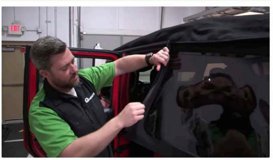
Now take the bottom plastic channel flap on the window and slide that into the body tub rail.
