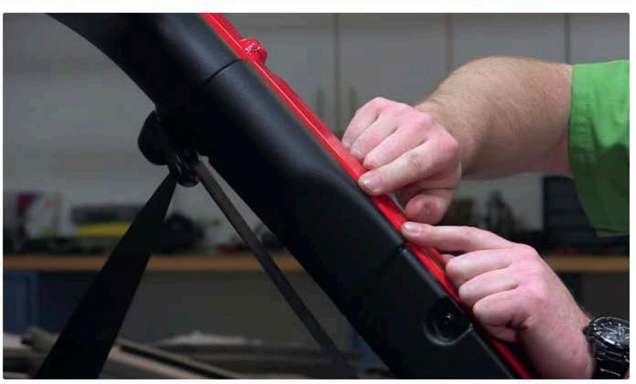
Use the T40 bolts to connect the sport bar brackets. These are marked right and left hand as well as which side goes up along with 2 locating pins to make sure the bracket goes in the exact right spot. Repeat this process for the driver side.
