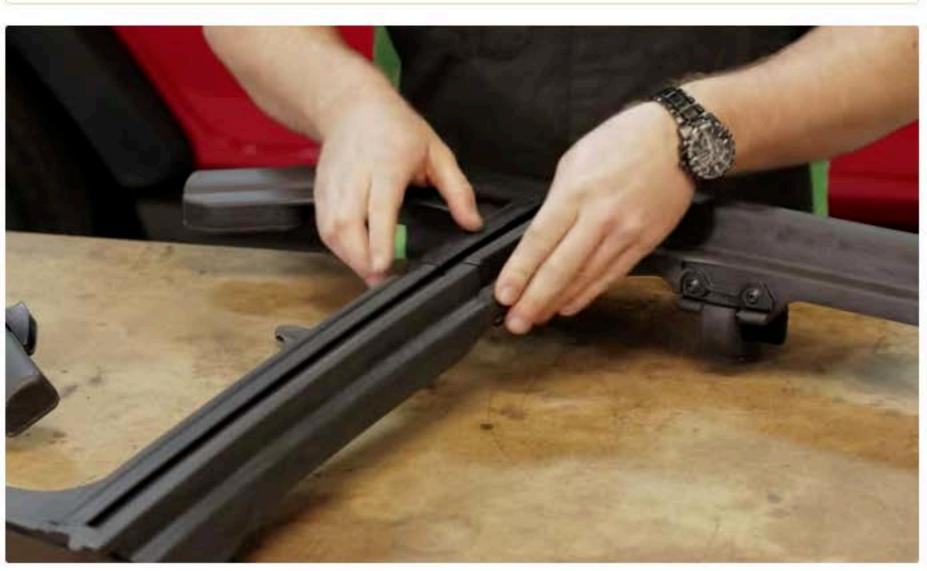
Attach tailgate bar brackets to rear body of tub next to the tailgate. Use one supplied T50 bolt.
