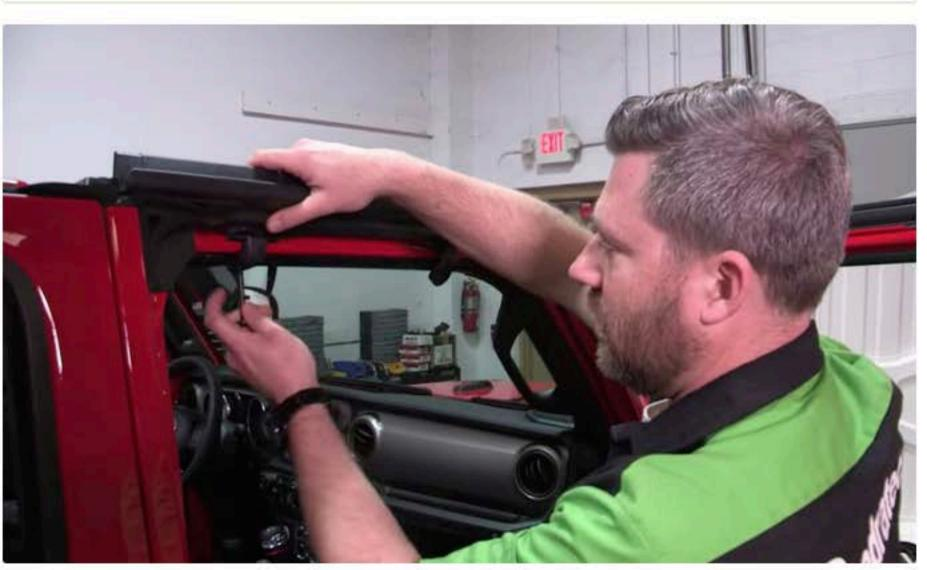
Same as with the front door surrounds, the rear door surrounds have notches that fit into the top of the sport bar. In addition there are a couple pegs on the bottom of the surround that fit into the belt rail of the Wrangler.
