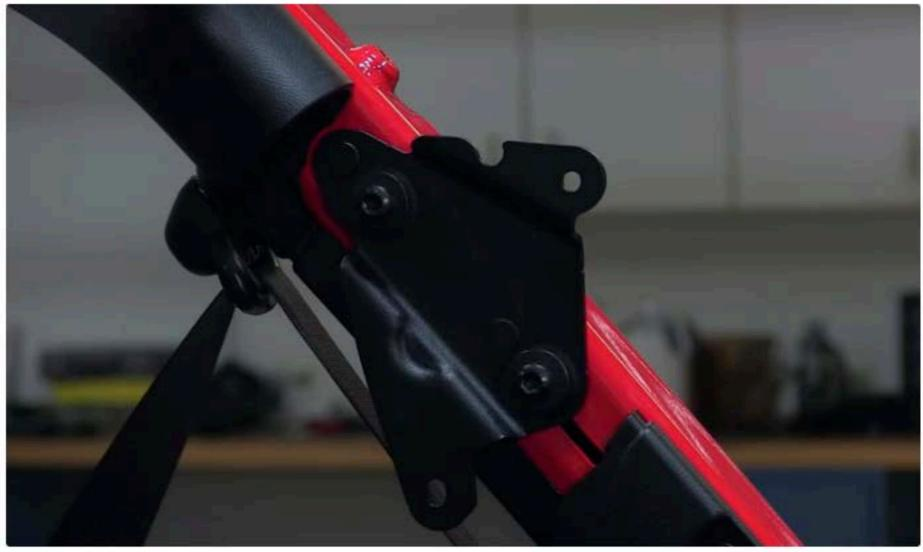
Next you can go ahead and install the door surrounds on the vehicle. Start with the front door surrounds. Place the bracket on top of the sport bar above the passenger side door, there are 2 notches that will drop into the holes on the top of the sport bar.
