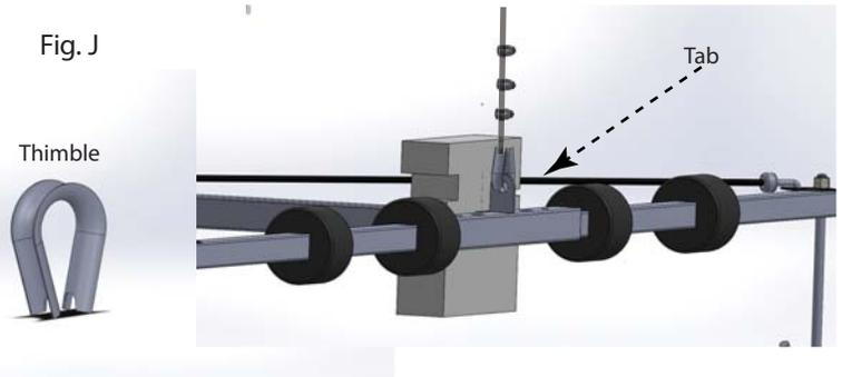
As shown in Fig. K, feed the cable through the hole with the thimble, install cable clamps loosely at first, in order to balance the frame. With the frame level on the floor pull the cable taut and secure the cable clamps in the order shown in figure K. Be careful to not over tighten these as they will strip. If they do become stripped or are suspect do not use them, they can be inexpensively obtained at any hardware store. Inspect these and all hardware before each use.
