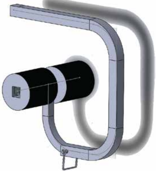
Fig. 7 Depiction of the assembled rear support. Should be assembled in steps after frame is assembled and needs to be fitted with care-through window.
