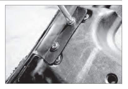
9. Raise top and bow assembly in upright position and lock header to windshield. With top loosely over bow assembly, reattach fabric to bows using screws removed in step 3. Fabric on rear bow wraps under bow from back to front of vehicle. Fabric on middle bow wraps over bow from front to back of vehicle.
