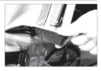
12. Insert tailgate bar into new rear window and install rear and side windows. Secure top above doors by inserting plastic retainer strips in door surrounds.
