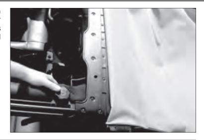
7. Place new soft top fabric on header with bottom side facing upward. With fabric draped over windshield, locate and align center notch on fabric and header. If necessary, use tape to hold fabric in place. Reattach top portion of header using screws removed in step 6.
