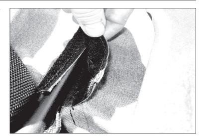
11. Insert rear corners of soft top into belt rail.
