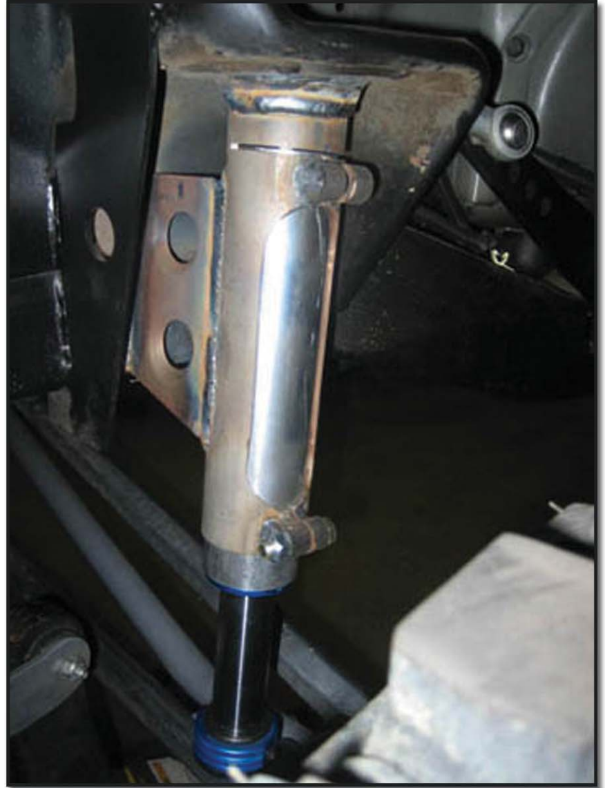
Air Bump Kit installation in progress
