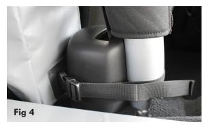
**3-**Buckle the E strap around the rear vertical roll bar, above the seat belt holder, without twisting the strap (Fig 3 and Fig 5).
