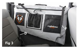
**2-**Buckle the D strap around the base of the rear vertical roll bar, without twisting the strap (Fig 3 and Fig 4).
