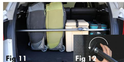
7-Rotate the rubber pads (Fig 12), if necessary, and move the handle back and forth until the Cargo Bar tightens snugly against the walls of the SUV cargo area.
