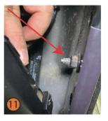
Step 6. Reverse steps 1 thru 3 to re-install your new tail light and proceed to the other side. FYI, You maybe have to back out this stock bolt (near the tail gate) before installing the new tail lights. (Photo 11)
